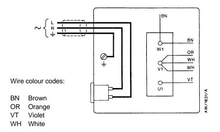
Figure 3 - Electrical supply connection, single-phase motors, 220-240 V 50 Hz, or 230-240 V 60 Hz
