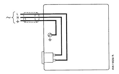
10. Check that the cable connections are correct, then refit the cover on the motor terminal-box.
