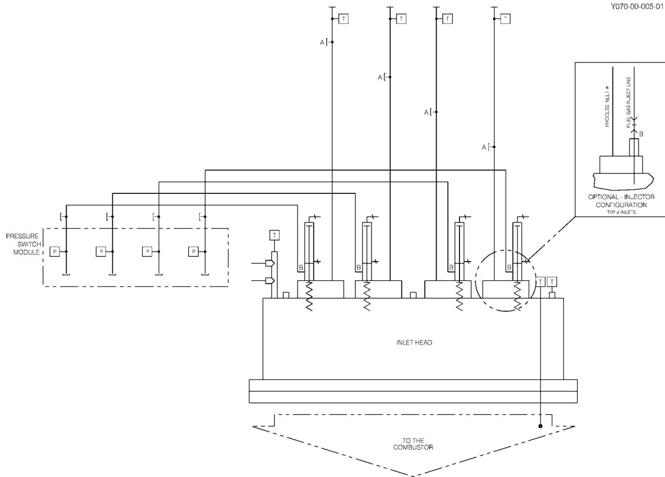
Figure 4 - Abatement system enclosure piping and instrumentation diagram (sheet 2): TCS inlet head
