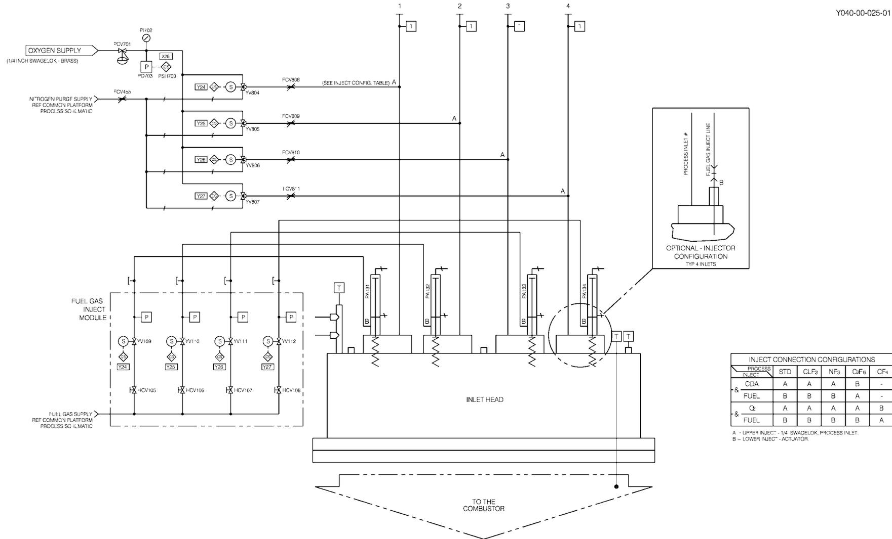
Figure 4 - Abatement system enclosure piping and instrumentation diagram (sheet 3): TPU inlet head
