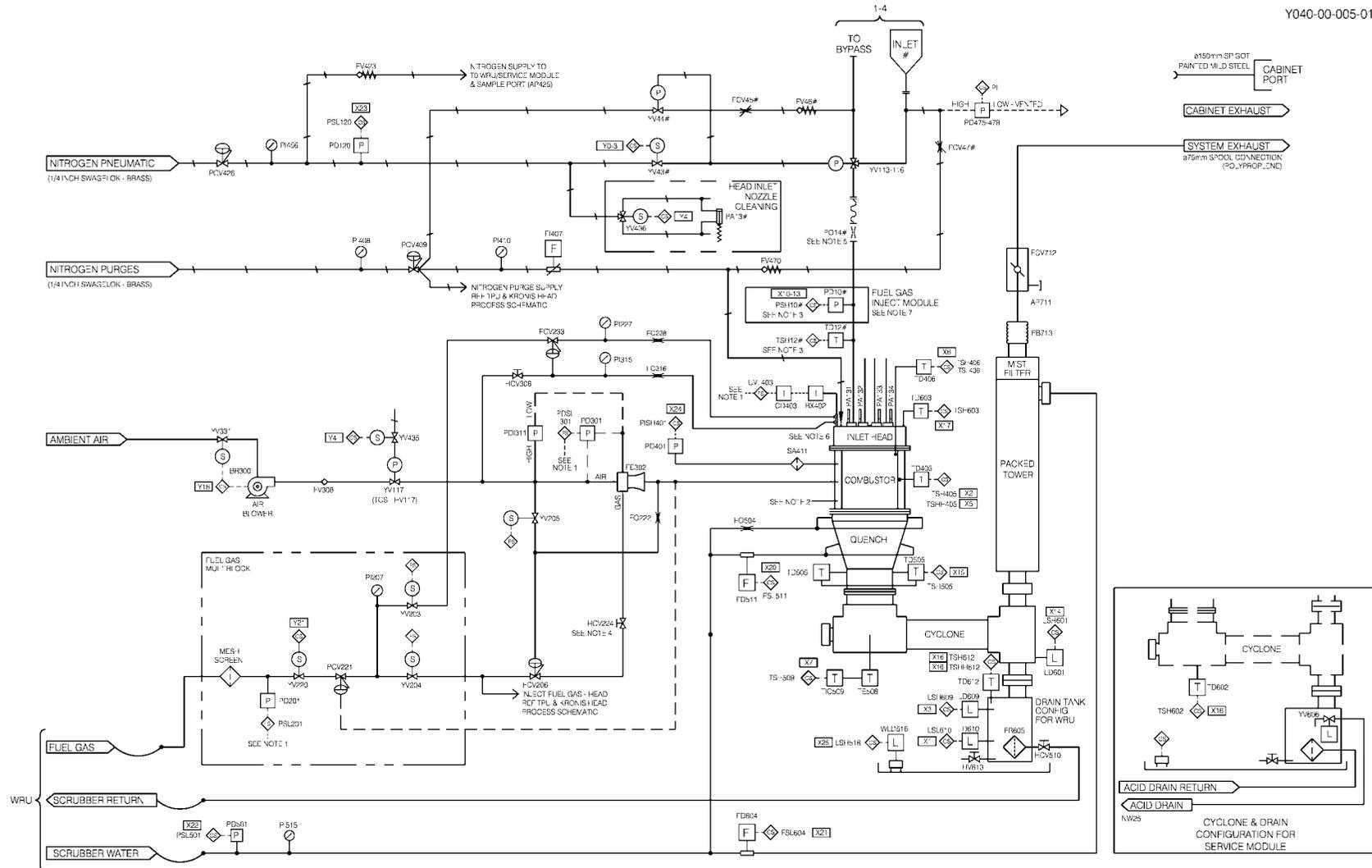
Figure 4 - Abatement system enclosure piping and instrumentation diagram (sheet 1): abatement system enclosure
