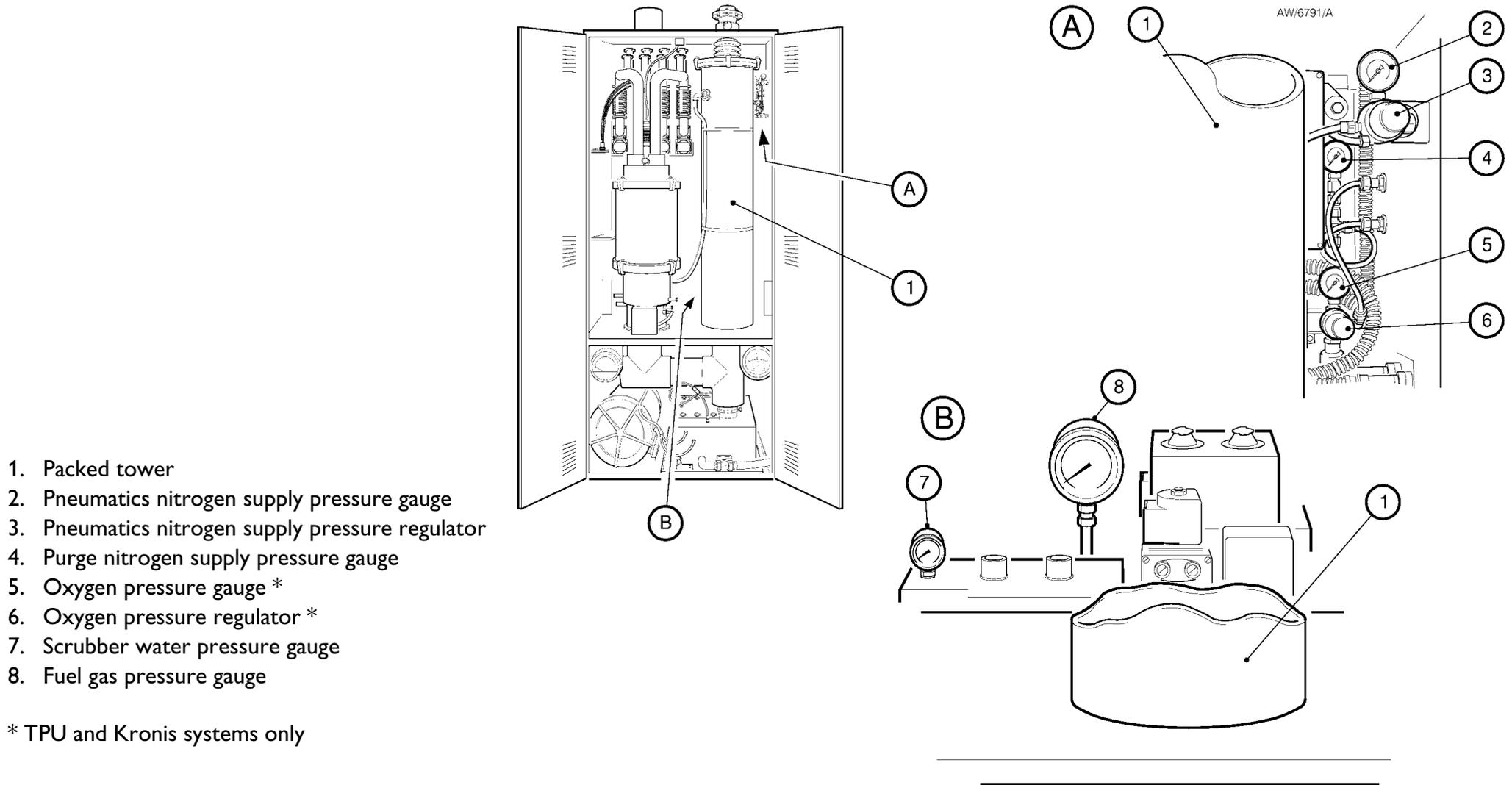
Figure 25 - Locations of the pressure gauges in the abatement system enclosure
