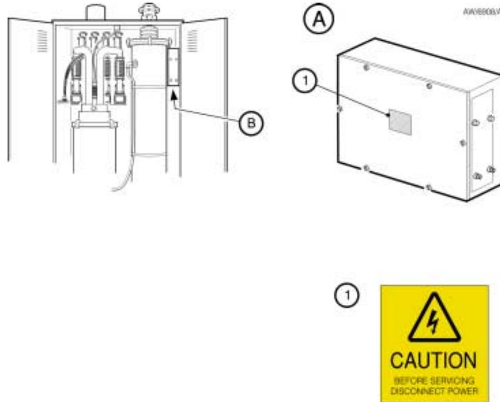
Figure A7 - Kronis TMS control unit warning label
