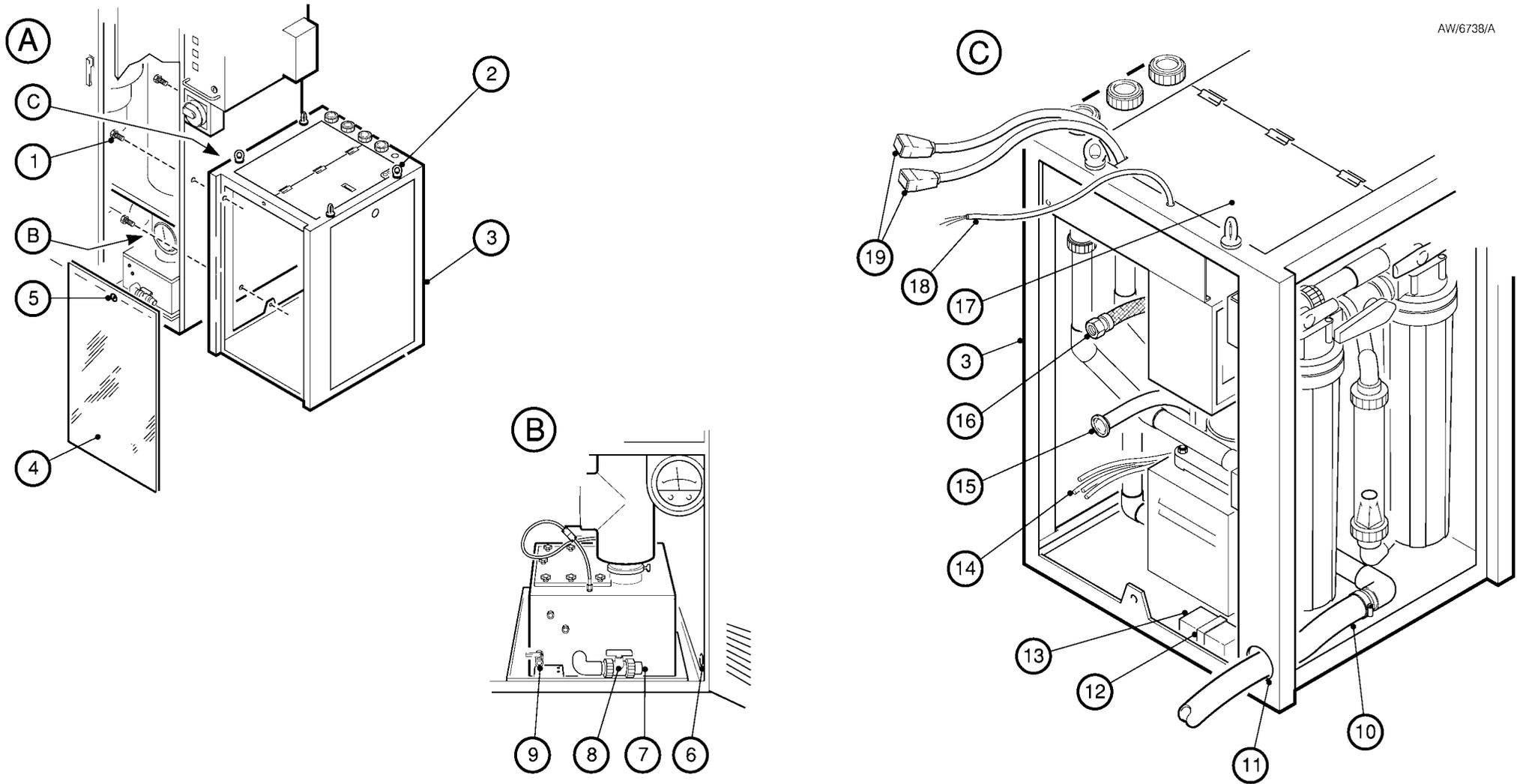
Figure 11 - Fit the WRU to the abatement system enclosure
