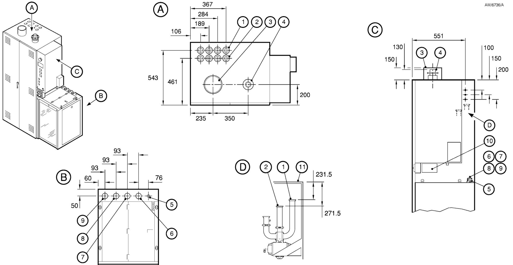
Figure 9 - Connection dimensions (mm)
