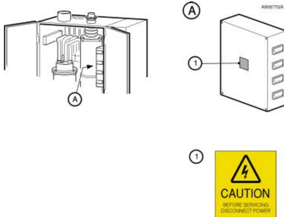
Figure A4 - TCS/TPU TMS warning label
