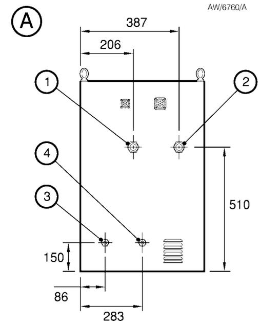
Figure A14 - Services Module connection dimensions (mm)
