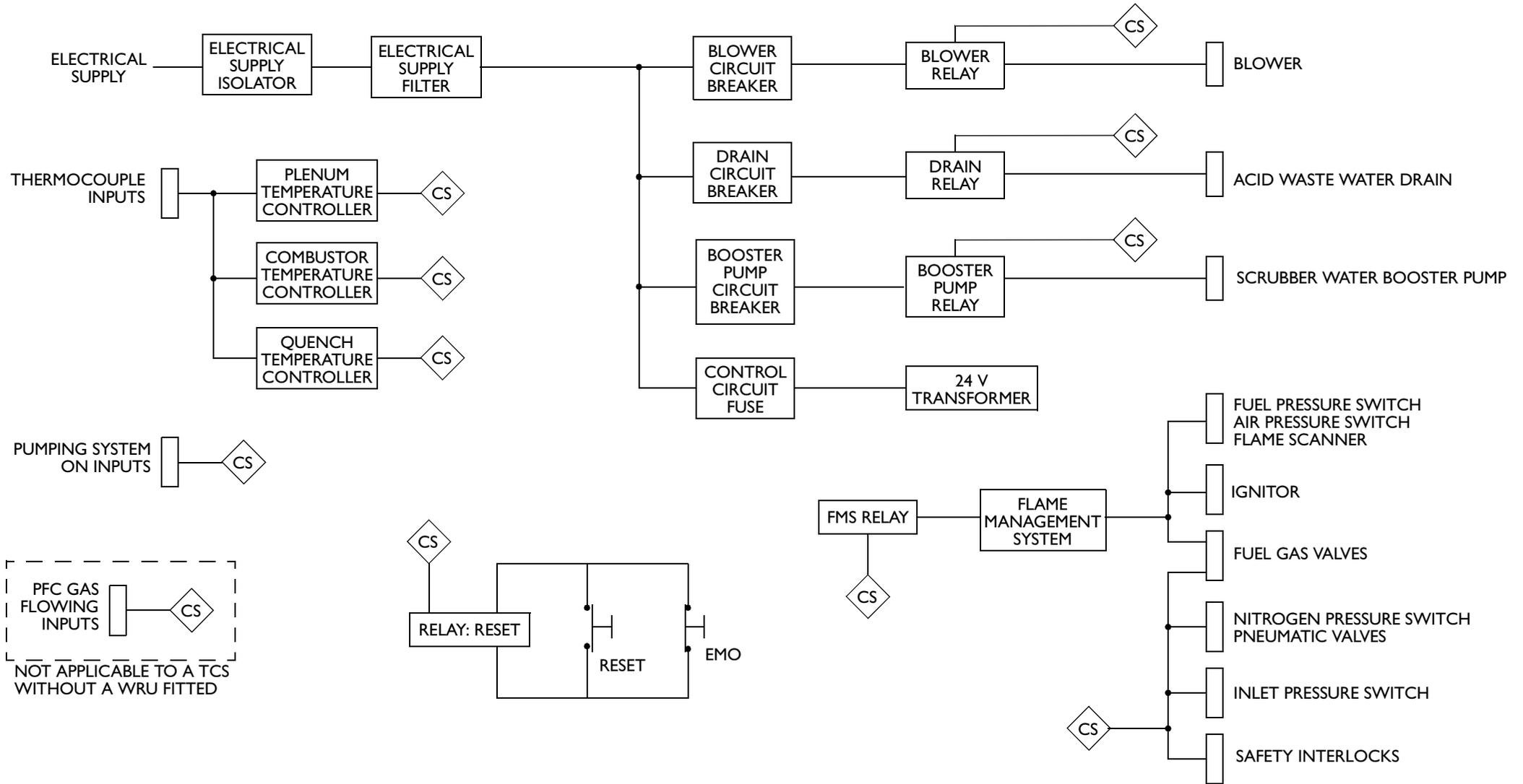
Figure 26 - Electrical block diagram
