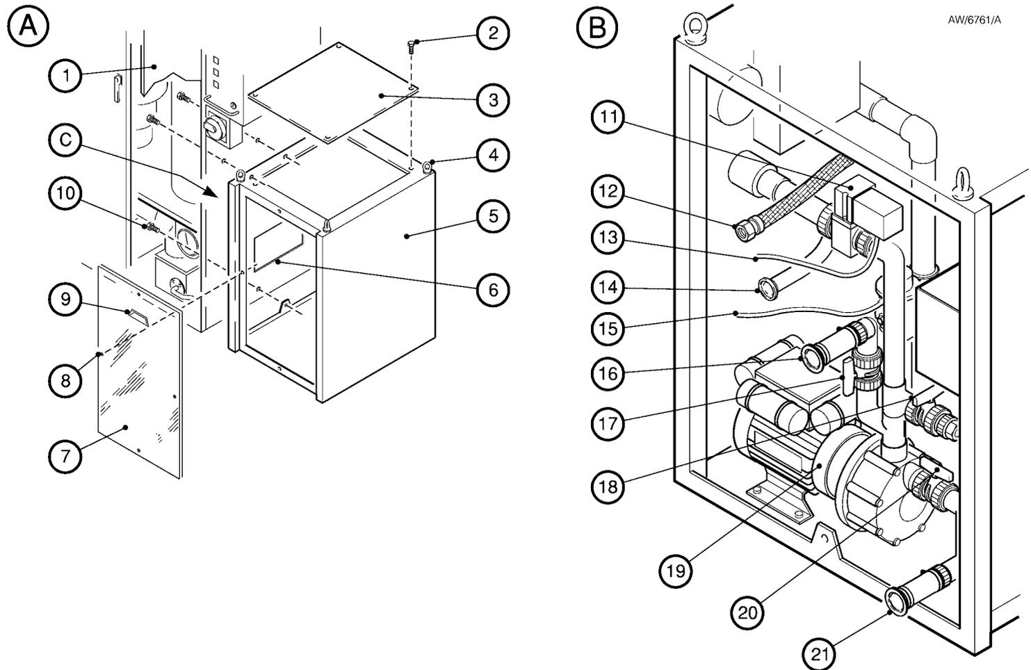
Figure A16 - Fit the Services Module to the abatement system enclosure
