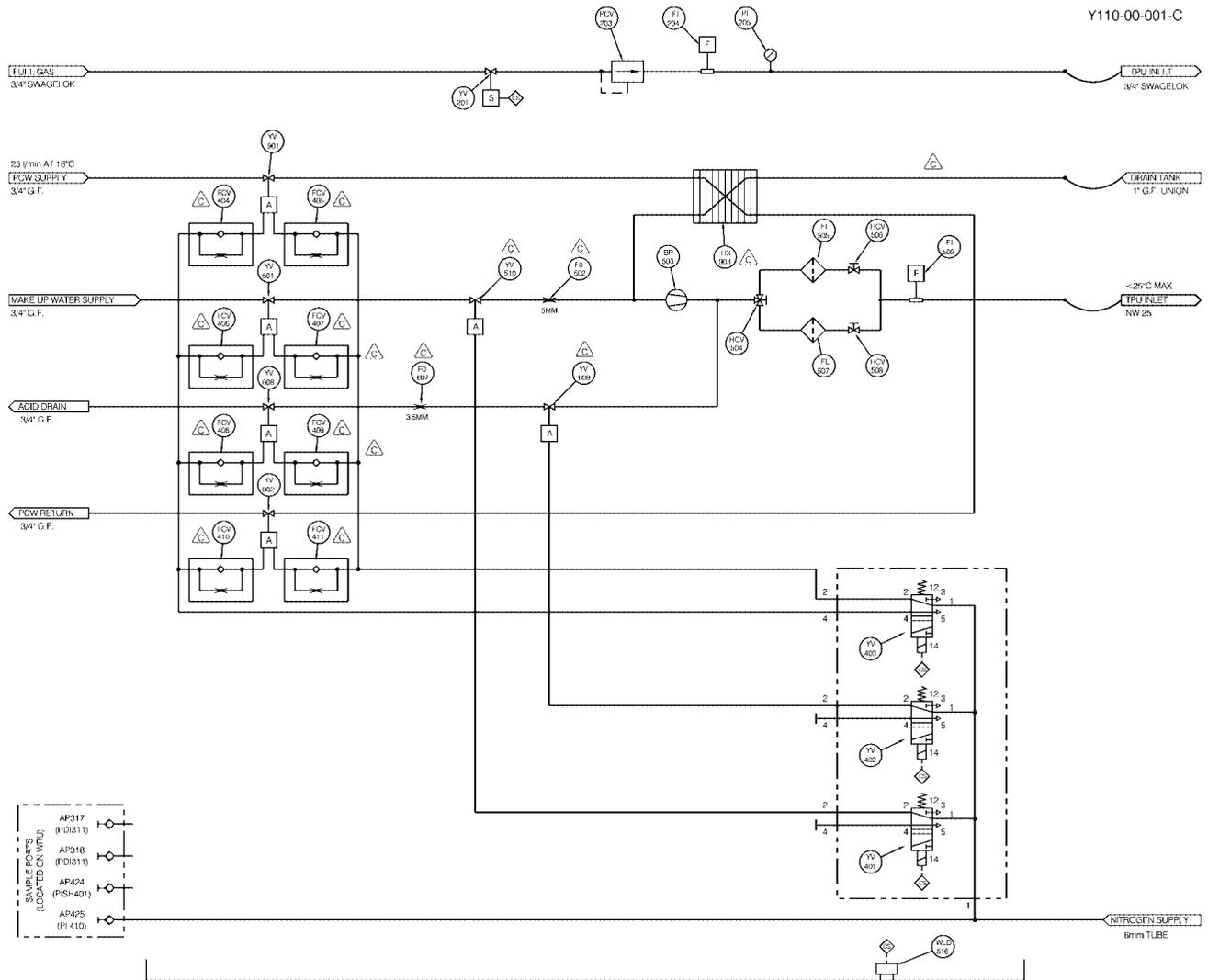
Figure 5 - WRU piping and instrumentation diagram
