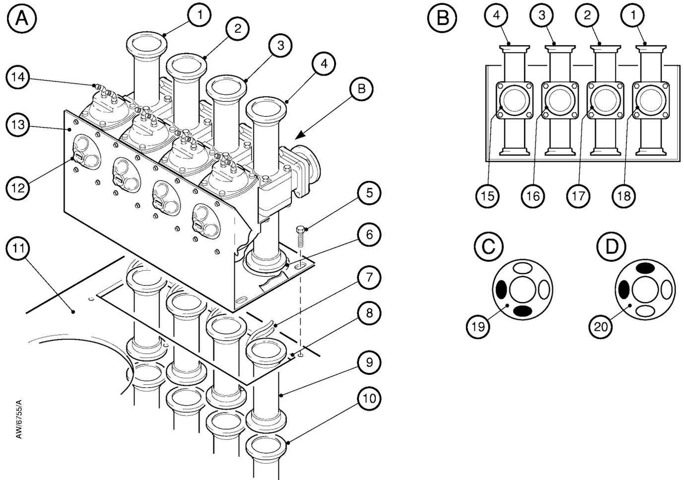
Figure A8 - Fit the Remote Bypass Module
