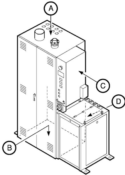
Note: The area above the WRU must be kept free for access: refer to [Section 3.4](#)
