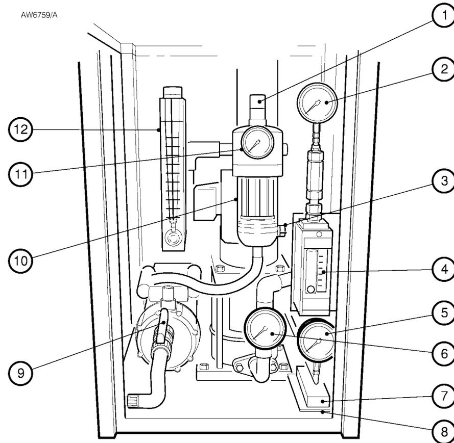
Figure A13 - Services Module controls and indicators
