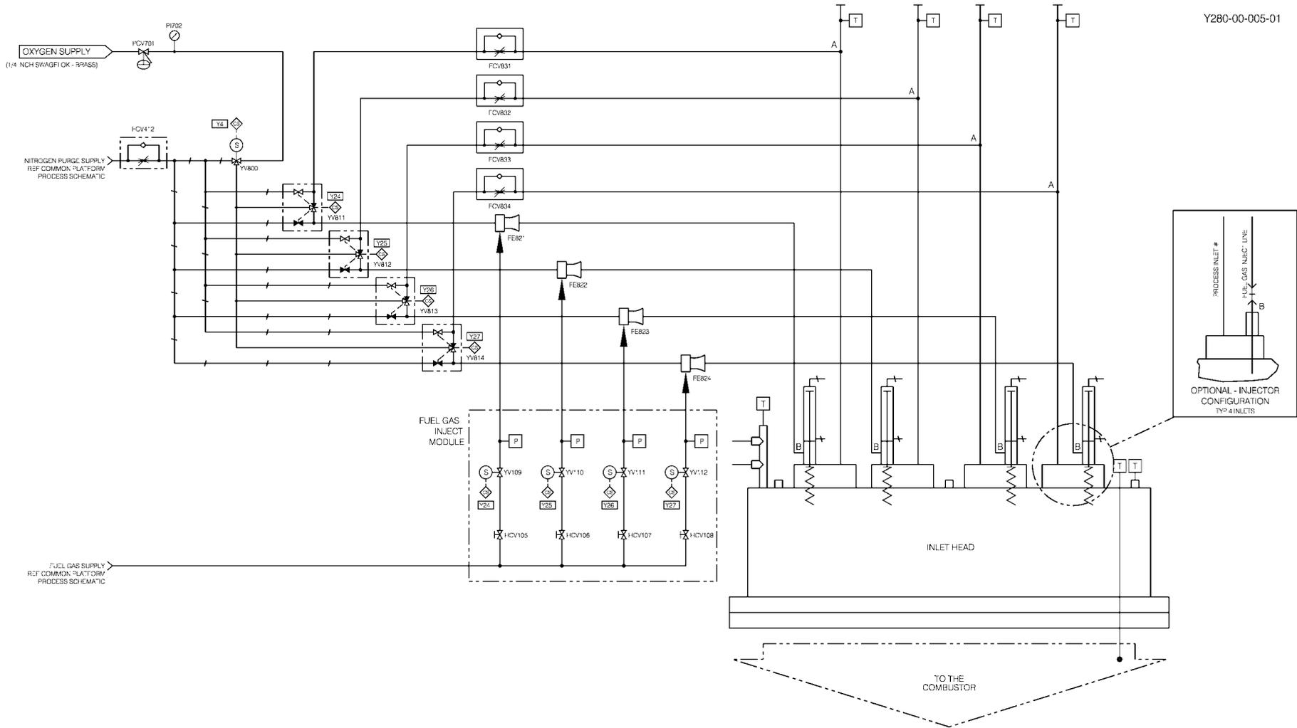
Figure 4 - Abatement system enclosure piping and instrumentation diagram (sheet 4): Kronis inlet head
