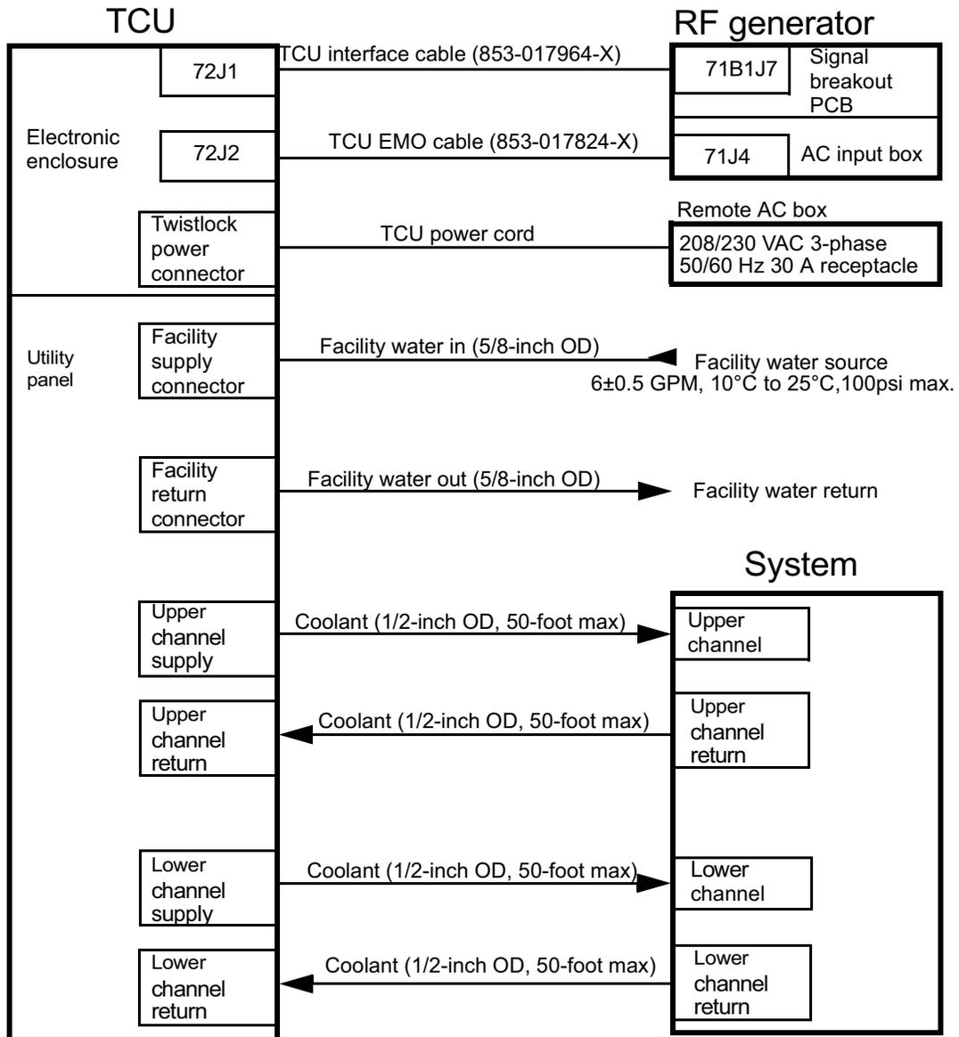
Figure 2-4. TCU Facility/Electrical Installation -Multi-chamber System/OEM
