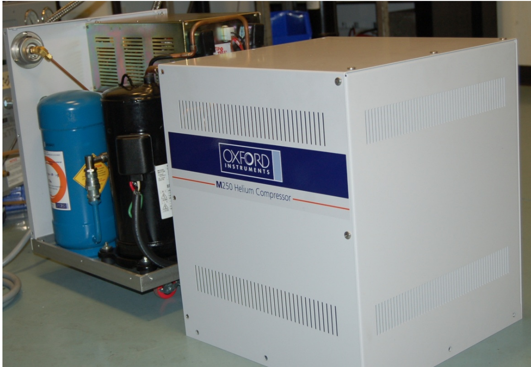
Figure 6 – Removal of Cover Panels
