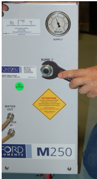
Figure 8 – Adsorber Aeroquip Nut Removal
