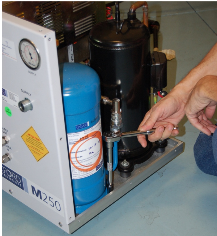
Figure 9 – Adsorber Chassis Screw Removal
