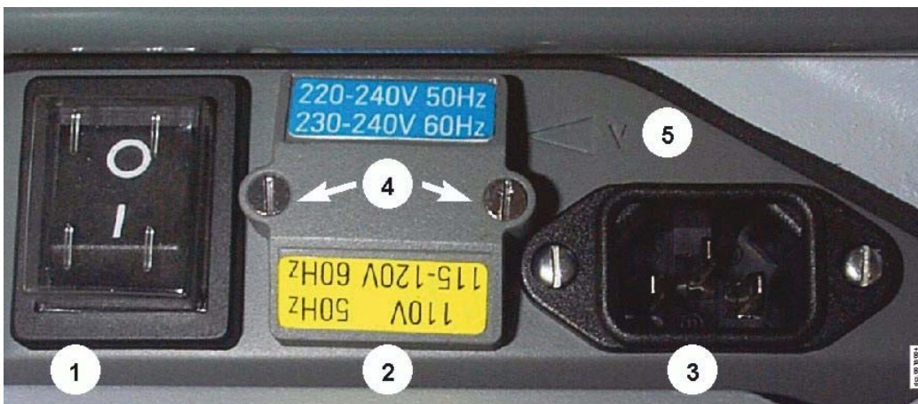
Figure 4 - Electrical interface: single-phase pumps
