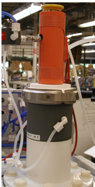
Figure 4-5: Type 20 inlet KF-40 flange
