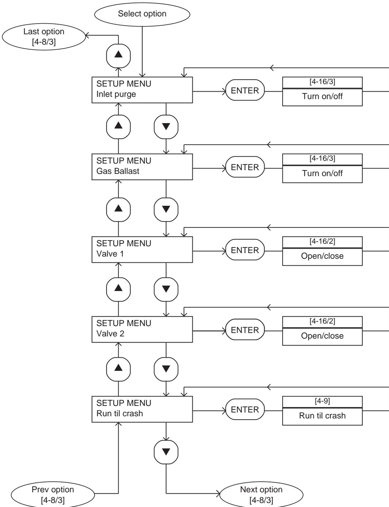
Figure 4-8 - Setup menu: sheet 2 of 3
