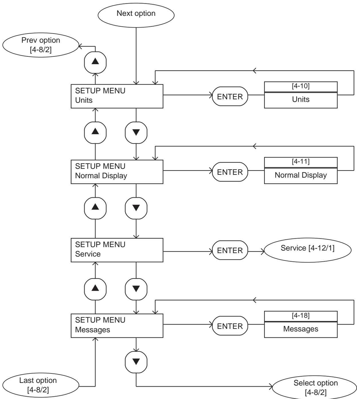
Figure 4-8 - Setup menu: sheet 3 of 3
