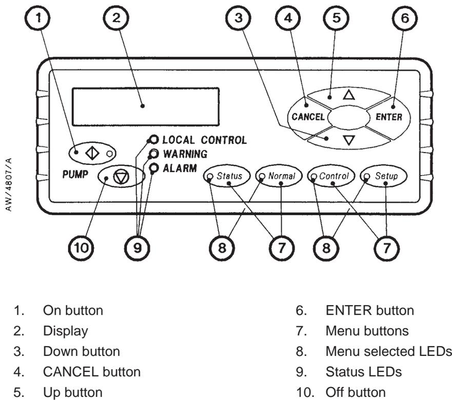
Figure 4-1 - Front panel of the Pump Display Module (optional accessory)
