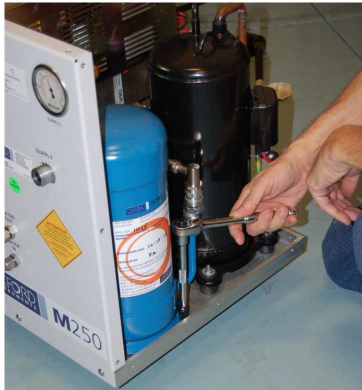
Figure 9 – Adsorber Chassis Screw Removal
