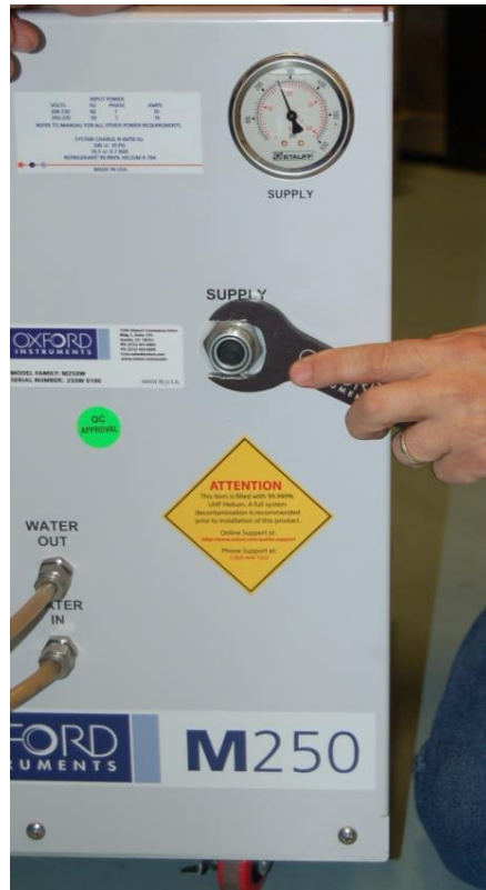
Figure 8 – Adsorber Aeroquip Nut Removal
