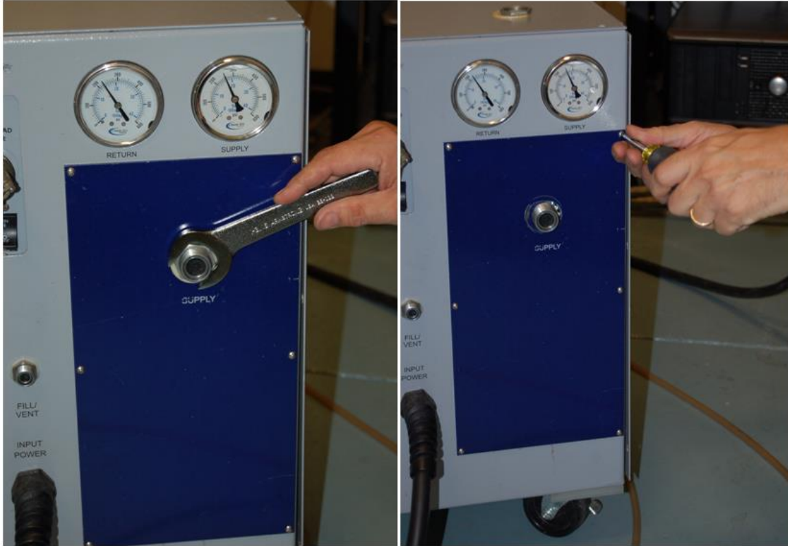
Figure 14 - Adsorber Aeroquip Nut and Access Panel Removal
