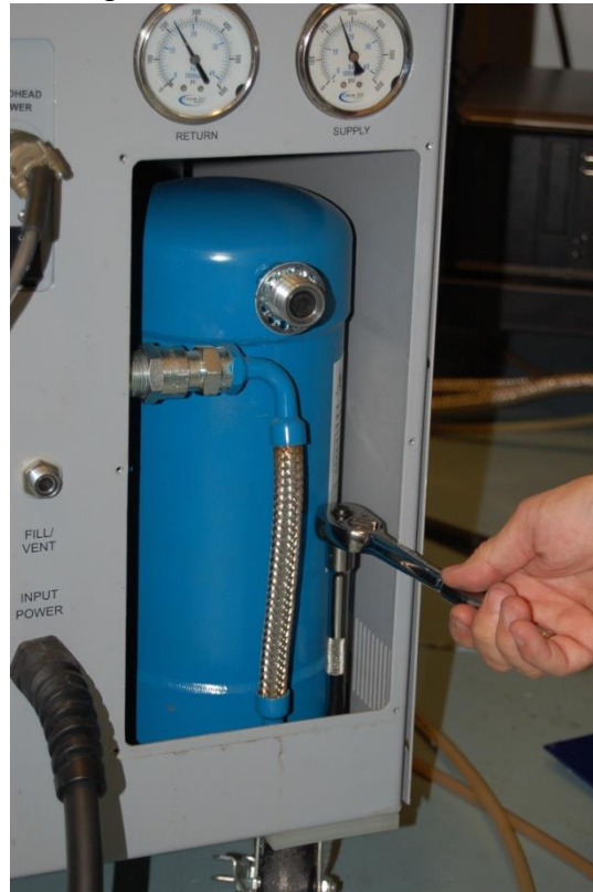
Figure 15 - Adsorber Screw Removal
